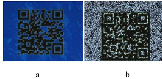
Figure 13. Arbitrary marks can be written on both (a) polished wafers coated with SiN and (b) textured silicon wafers coated with SiO<sub>2</sub>. The black marks are much more readable on the textured than lighter marks.
