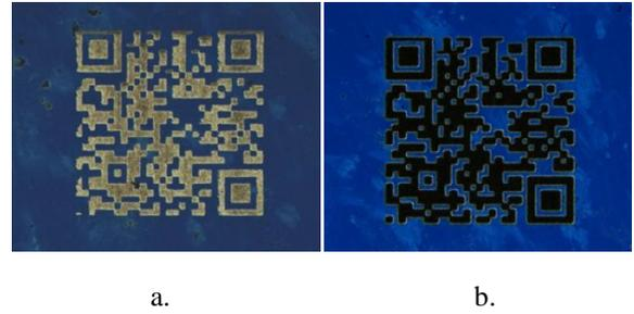
Figure 7. Two identical patterns made with different process parameters demonstrates the stark difference between (a) removal of the SiN layer and (b) marking/darkening the silicon beneath.
